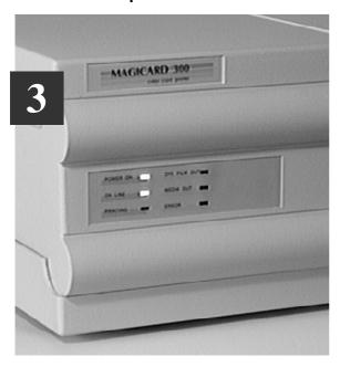
Switch ON. The indicators should all flash and the motors run briefly. Finally, the POWER ON and ON LINE indicators will remain ON..
